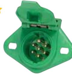
Color-fast green glass-filled plastic insures quick identification. Spring-loaded door is marked 'Trailer ABS' to further lessen any chance of misconnection. Mounting holes on the flanges are oval, .488" x .328" (12.4 x 8.3mm), 2.93" (74.6mm) on centers. Mounts through 2" (50.8mm) diameter hole.
