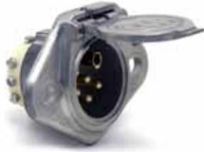
Diecast housing, polarized ground terminal, insulated. Replacement for ISO 3731-1976 (E) road vehicles, type 24S (supplementary). Contact pins: one spring-grip female, and six solid male. Mounting holes on the flanges are oval, .488" x .328" (12.4 x 8.3mm), 2.93" (74.6mm) on centers. Mounts through 2" (50.8mm) diameter hole. Mates with Cole Hersee 11100-02 and 11100-01 plugs.
