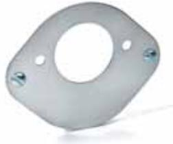
Heavy duty adapter provides secure seating for attachment of sockets, and permits installation of fuse/breaker block or terminal block in the rear. Mounting holes 5/16" (7.9mm) diameter, 4 1/2" (114.3mm) on center. Mounting hardware included.
