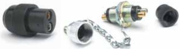
Screw-on cap protects the socket from dirt and moisture when not in use. Polarized for proper mating of circuits. Includes one 1102-F plug. Mount in 45/64" (17.9mm) diameter hole in panels up to 3/8" (9.5mm) thick. Plated steel cap and housing.
