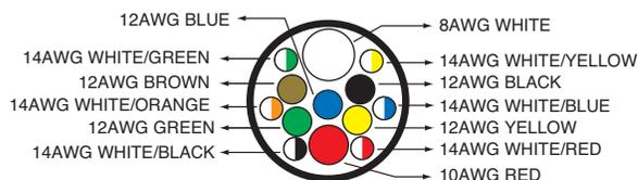
Will not crack or stiffen at -70°F (-57°C). One 8AWG, one 10AWG, five 12AWG and six 14AWG wires, 100% electrical copper for maximum conductivity.
