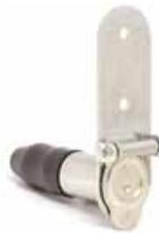
Brass contacts and terminals. Accepts up to 6AWG cable. Corrosion-resistant plated steel housing. Stainless steel spring on the cover locks the plug in place, closes securely to protect the contacts. Rubber boot protects terminals and cable connection. Integral mounting bracket has two .218" (5.6mm) diameter mounting holes, 1.25" (31.8mm) on centers.
